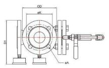
**NOTE:** To allow for maintenance while installed, the Model C-EL shall have a free space of 2/3rds its length (L2) at the valve trim side.
